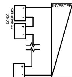
DC/DC CONVERTERS ARE ALL RUN IN SERIES (FIXED SOURCE CIRCUIT VOLTAGE DC/DC CONVERTERS)
