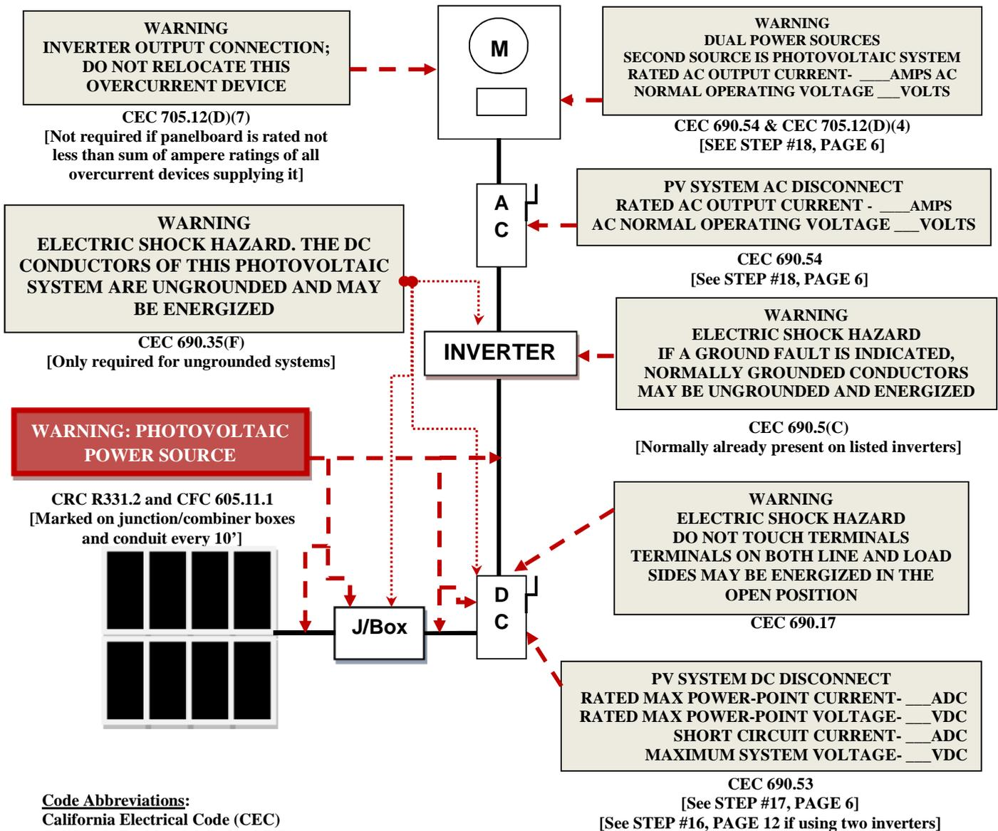
Informational note: ANSI Z535.4 provides guidelines for the design of safety signs and labels for application to products. A phenolic plaque with contrasting colors between the text and background would meet the intent of the code for permanency. No type size is specified, but 20 point (3/8") should be considered the minimum.
